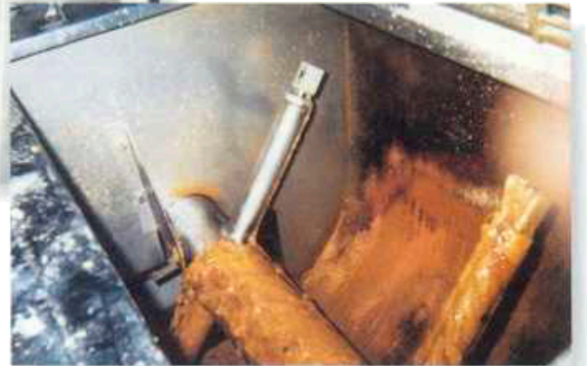
Figure 3: Partially cleaned mixer in a sweets factory
