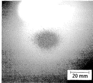
**Figure 5: Roughened aluminum surface**
